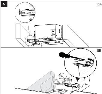
Secure the suspension bracket (C) to fan housing using screw (CC) (included). Secure suspension brackets (D, E) with screws (BB) (included).
