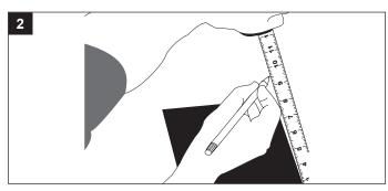
3. If this fan is not replacing an old fan, be sure to cut a 9-1/4 in. x 9-1/4 in. opening for the fan housing.
