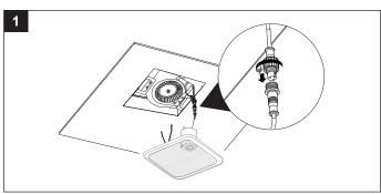
Attach grille by pinching mounting springs and insert into narrow rectangular slots in the fan housing.
