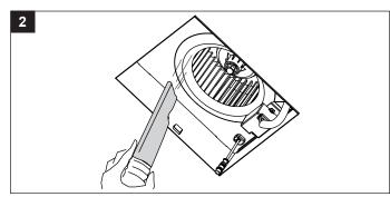
3. Dampen cloth with dust detergent, wipe the fan housing and wipe dry with a cloth.
