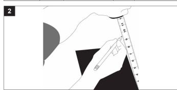
3. If this fan is not replacing an old fan, be sure to cut a 7-1/2 in. x 7-5/32 in. opening for the fan body (A).
