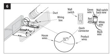
7. Connect a 4 in. circular duct and vent to the outside. Secure it with duct tape or clamp.
