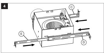
5. Position fan housing so edge of fan is flush with sheetrock. Do not flush mount housing with joist.
