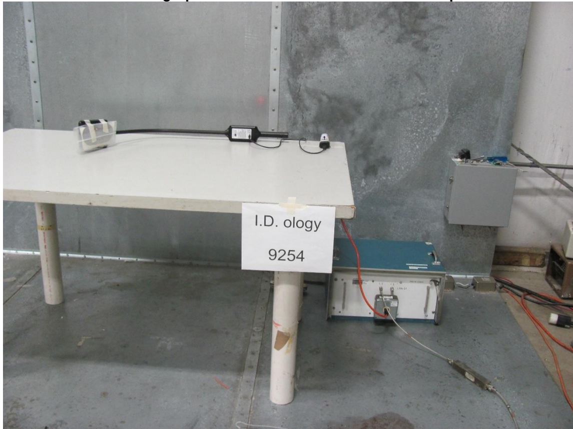
Photograph of Conducted Emissions Test Setup
