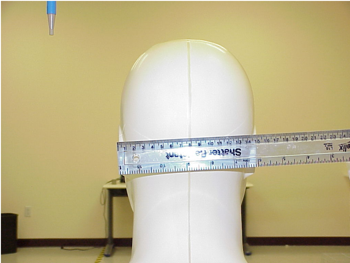
Photo 9. Photo to demonstrate 15 cm Z-axis head phantom
