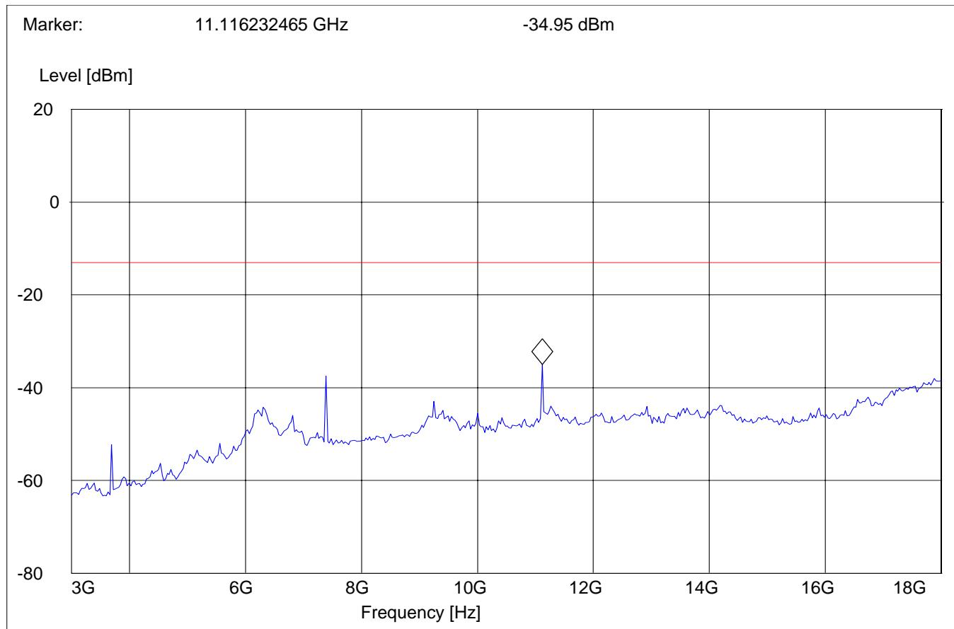
**RADIATED SPURIOUS EMISSIONS****Tx @ 1880.0MHz: 1GHz – 3GHz**
