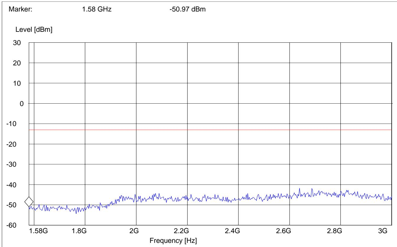
**RADIATED SPURIOUS EMISSIONS (GSM-850)****Tx @ 824.2MHz: 3GHz – 9GHz**
