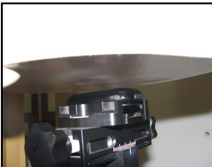
Figure 9.11 Muscle SAR Test Setup -- 15mm Distance Position --
