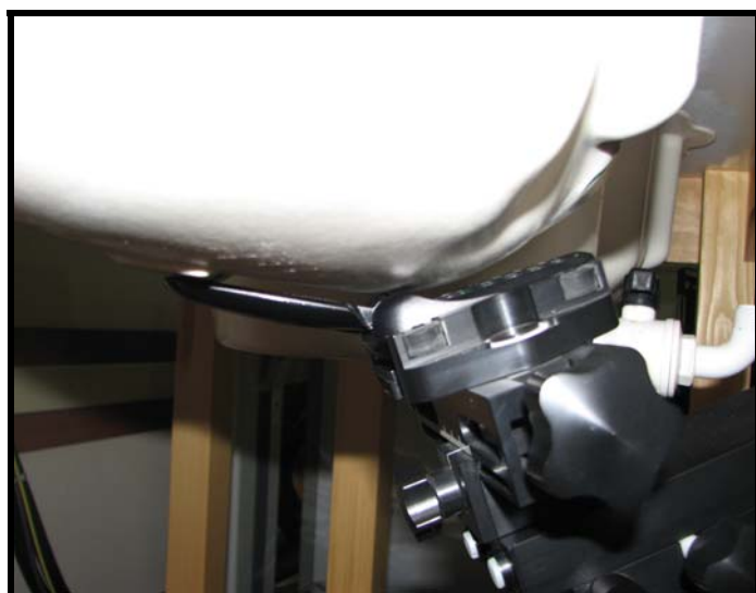
Figure 9.1 Right Head SAR Test Setup -- Cheek / Touch Position --
