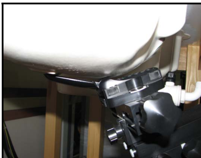
Figure 9.7 Right Head SAR Test Setup -- Cheek / Touch Position --
