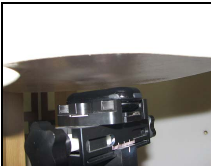
Figure 9.5 Muscle SAR Test Setup -- 15mm Distance Position --
