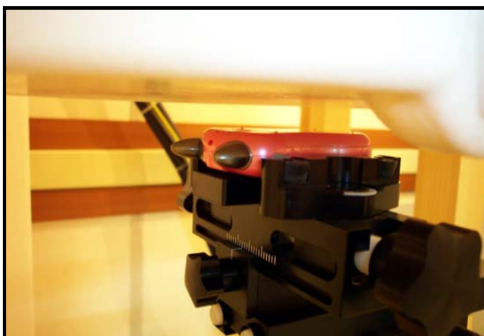
Figure 9.5 Muscle SAR Test Setup -- 15mm Distance Position --
