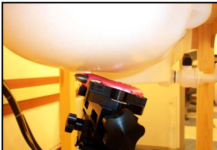
Figure 9.2 Right Head SAR Test Setup -- Ear / Tilted Position --
