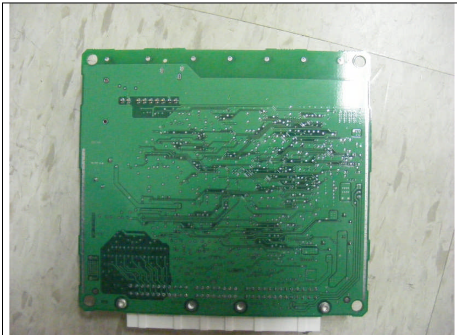
Bottom View of Main-board
