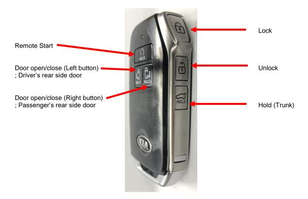
You can lock, unlock, open trunk and so on your vehicle with this remote transmitter.
