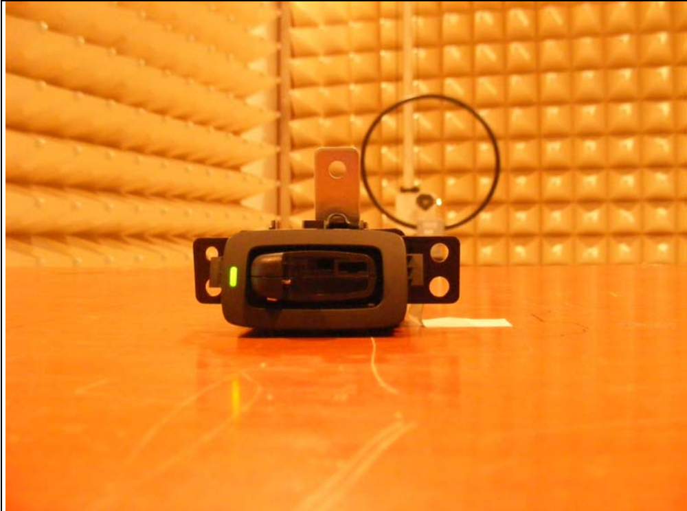
Photo of Field Strength & Spurious Emission Test
