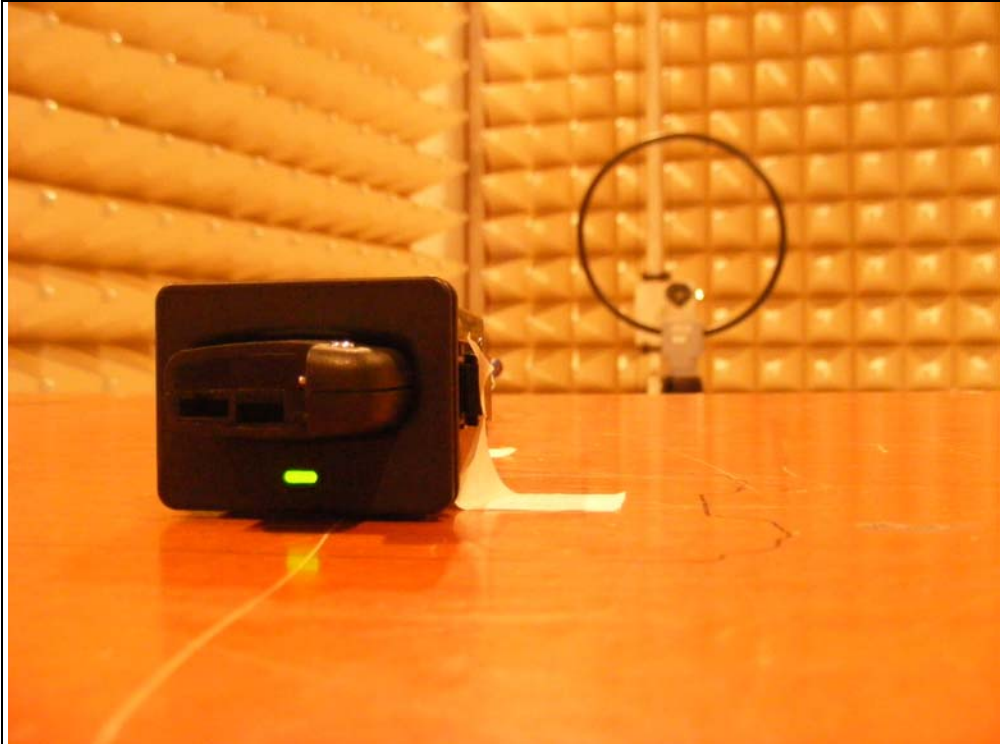
Photo of Field Strength & Spurious Emission Test
