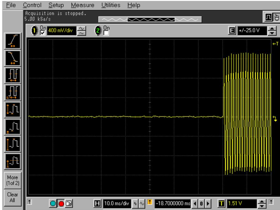
Test Plots for channel spacing 12.5KHz. EUT power setting: Maximum
