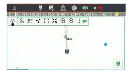
After setup the station, you can enter the measurement interface  $\Re$  for point measurement. The measurement interface is composed of five parts from top to bottom: status bar, information bar, Settings, toolbar and view.
