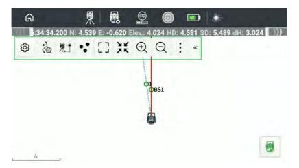
The display and order of the tools can be set in the measurement Settings. The default display tools include [Survey information], [Survey method], [Points], [Full], [Center], [Zoom in], and [Zoom out]. The default not display tools include [Redraw], [One-click Find], [Hide/show data], [Hide/show base map], [Delete previous point], and [Edit previous point]. The right side of the toolbar has [More functions] by default, and the far right side is the button to collapse and expand the toolbar.
