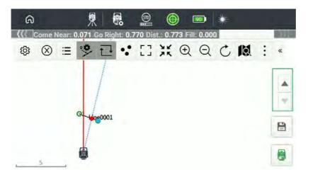
Click the survey button 🖲, after the stakeout is completed, the Save button 🗎 will
