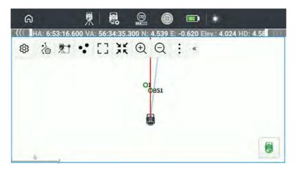
The icon of the total station is the position of the instrument, the red line is the direction of the station, and the blue line is the direction of the instrument. Point, line, and base map data can be displayed on the view. The scale \_\_\_\_\_ is displayed in the lower left corner of
