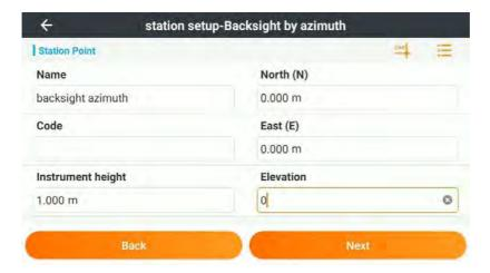
2. Enter the backsight azimuth to perform the backsight measurement
