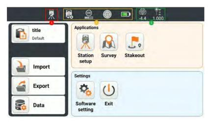
The title bar is divided into three parts: left, middle and right, the left is the station setup, the middle is the instrument setting, and the right is the prism setting.
