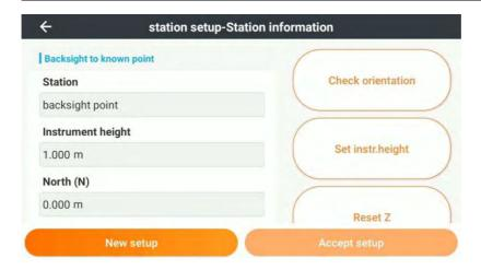
[Check orientation]: Select a known point for backsight measurement to verify that the current station is correct. If the current orientation of the station is wrong, the theoretical azimuth can be assigned to the actual measured direction to obtain a new station.
