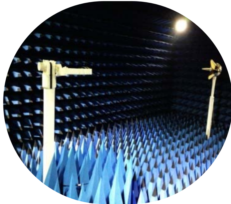
7m*4m*3m Anechoic Chamber
