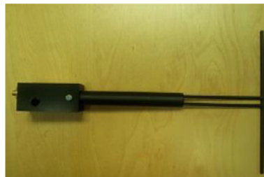
Figure 1 – MVG COMOSAR Validation Dipole
