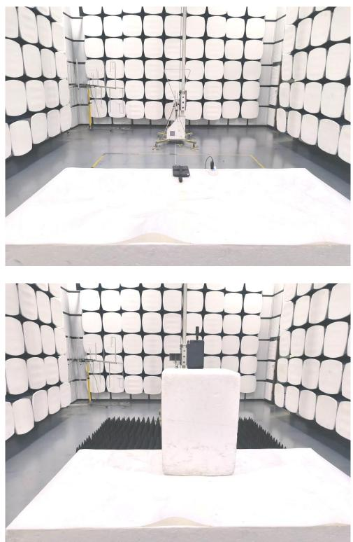
1.1. Photo of Radiated Emission test
