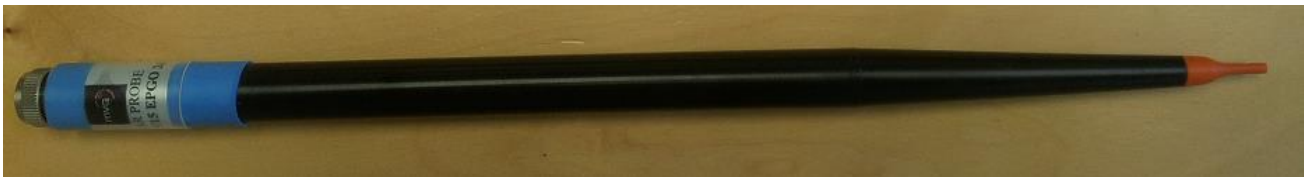
Figure 1 – MVG COMOSAR Dosimetric E field Dipole
