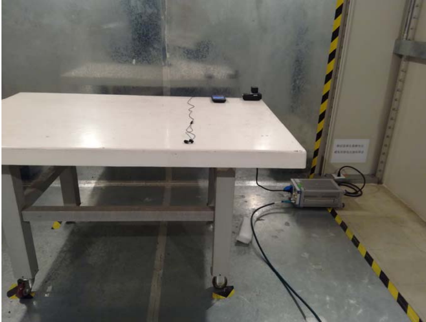
Conducted Emissions (Side View)
