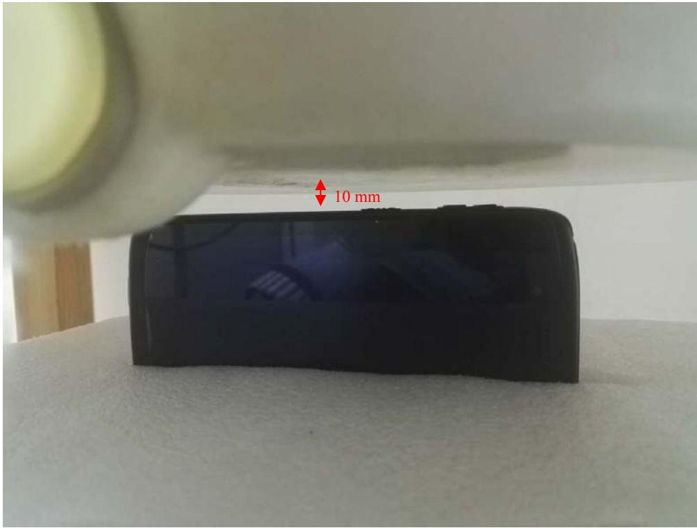
Body-worn Right Setup Photo (10mm)
