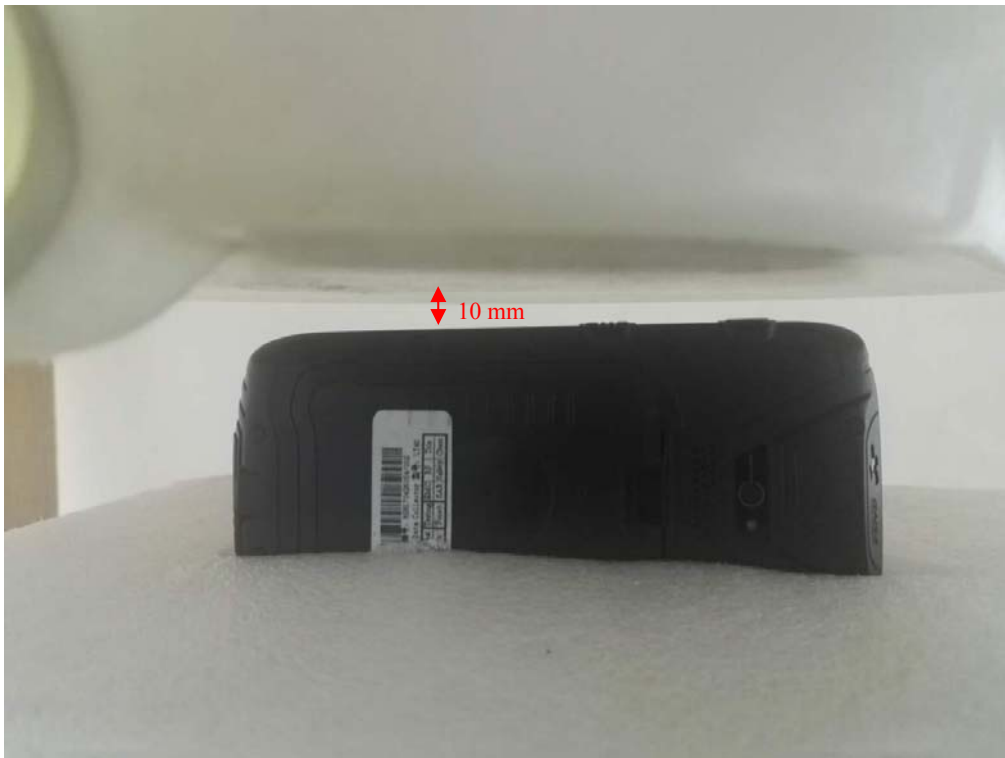
Body-worn Left Setup Photo (10mm)
