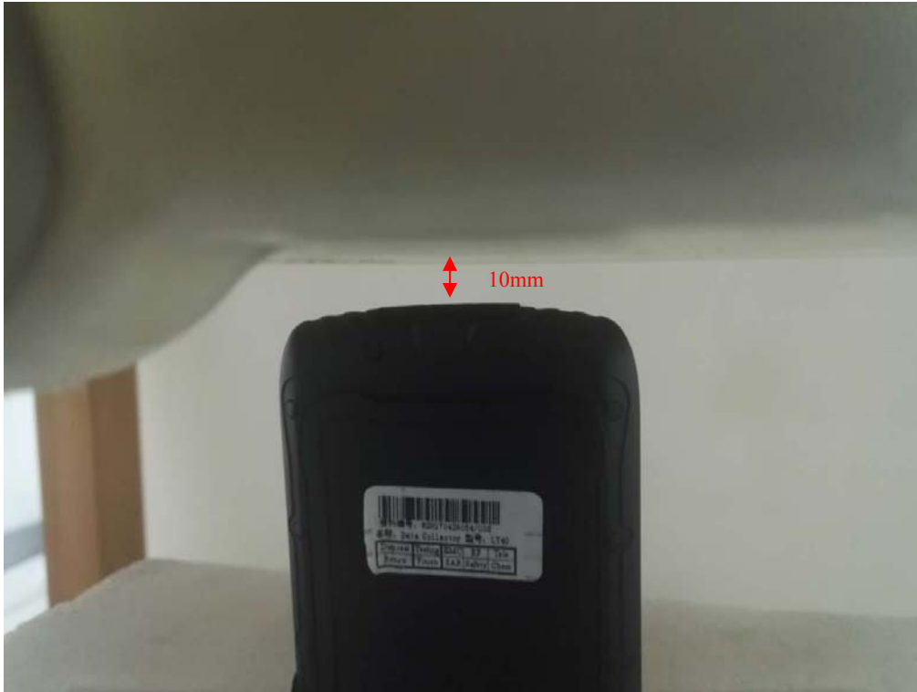
Body-worn Bottom Setup Photo (10mm)
