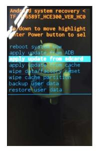
8.Select[update.zip], press power button to confirm and start the ARM11upgrade, waiting to progress bar has completed.
