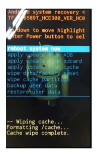
4.Clear users data:select[wipe data/factory reset],press the power button to confirm.
