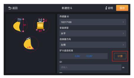
Measure S2 (vertical distance between the tilt axis and the top of the bucket at this horizontal attitude )
