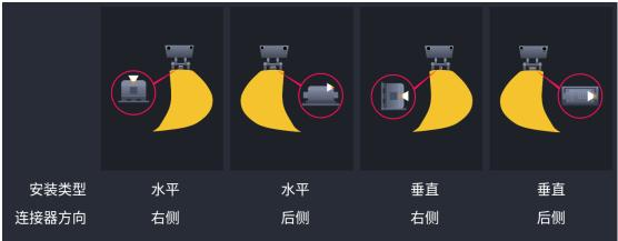
After configuring the basic information of the tilt bucket, adjust the left and right and rear directions of the tilt bucket, and click the [calculation] button to calibrate the tilt bucket sensor
