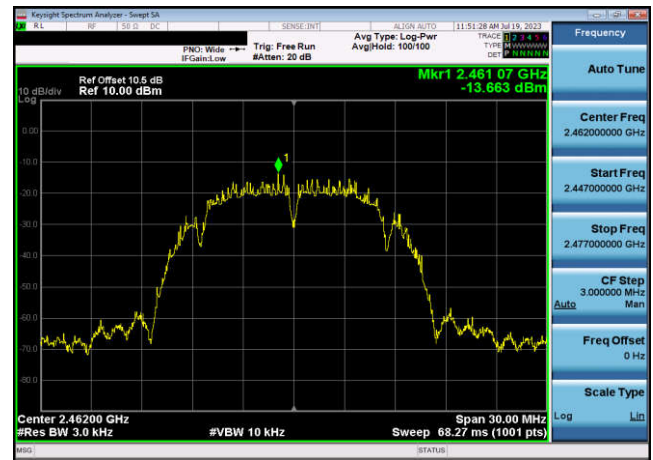
Power spectral density-802.11b ,2462MHz,Ant2
