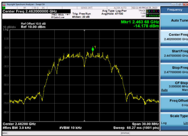
Power spectral density-802.11b ,2462MHz,Ant1
