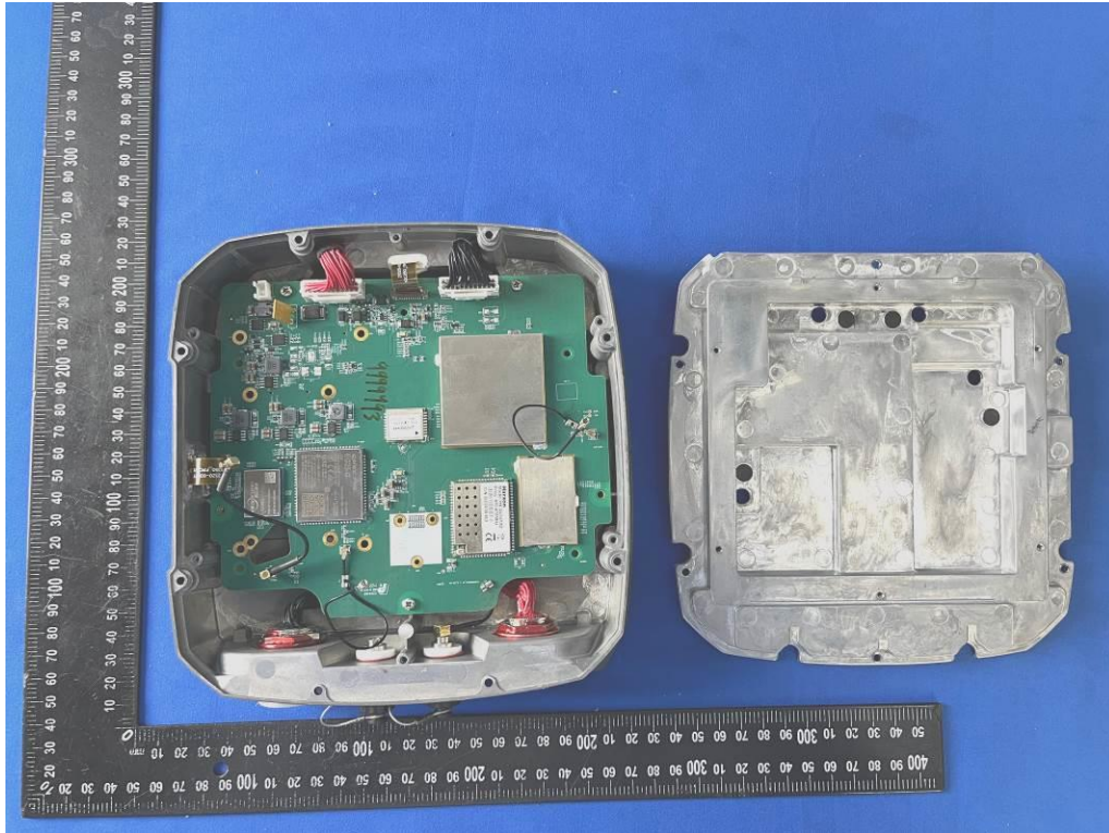
Internal view(PA-3 SE)
