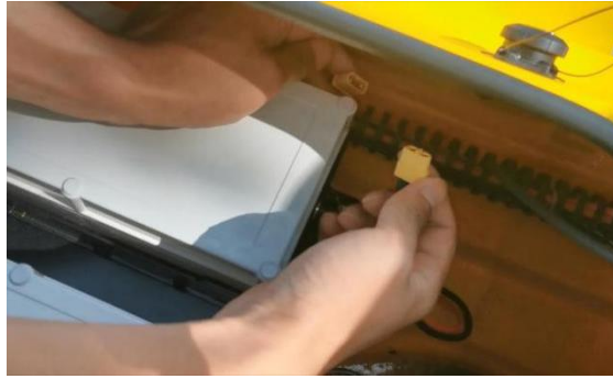
Figure 2-5 Connect battery-powered interface
