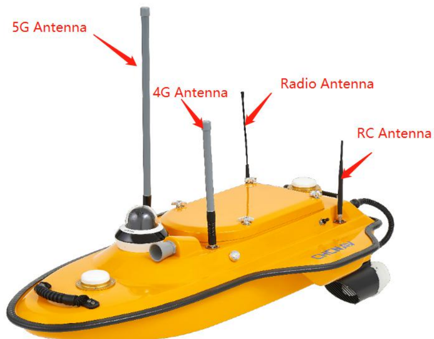
Figure 2-4 Install the accessories on the boat
