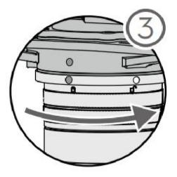
Rotate the GNSS antenna clockwise to the antenna bracket and tighten it. Connect the other end of the GNSS feeder to the GNSS interface of the AA450.
