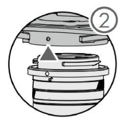
Rotate the AA450 SkyPort interface to the locked position (red dots align red dots) to be fixed.
