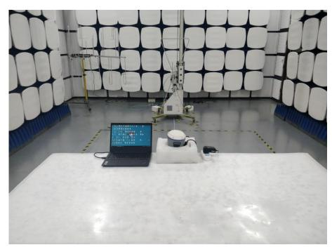
5.2.Photos of Conducted disturbance at mains terminals test
