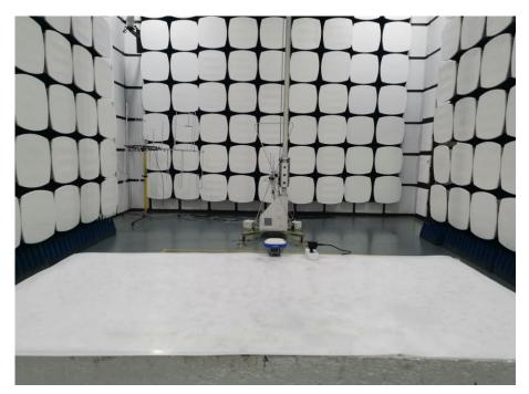
Photos of Radiated Emission Test (In Semi Anechoic Chamber above 1GHz)
