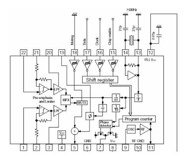
• FM oscillation section oscillates with 7.6 MHz Xtal frequency, by the PLL modulation method, generates 19 kHz and FM bands of frequency which is required for FM frequency transmission.
