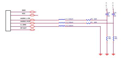
• Stereo L, R signal comes from MP3 player through L11, L12. This signal is regulated by resistor R1, R3. Then this Stereo L,R signal is forwarded to Pin 22 and 1 of BH1417F through C24 and C25.
