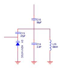
• This VCO(voltage controlled Oscillator) is Frequency tuning section. VCO tunes the voltage precisely, makes the RF output frequency to the frequency that the user sets, and fixes it.
