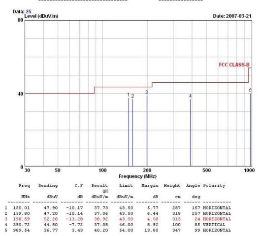
Remarks: C.F (Correction Factor) = Antenna factor + Cable loss - Preamp gain
