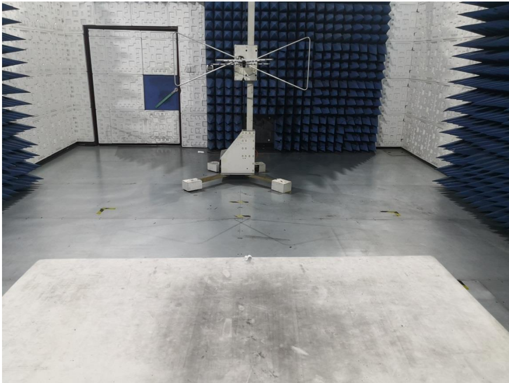
RADIATED EMISSION TEST SETUP ABOVE 1GHz
