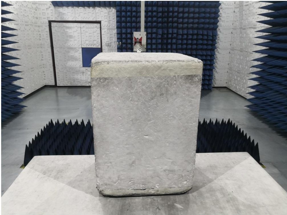
RADIATED EMISSION TEST SETUP ABOVE 1GHz
