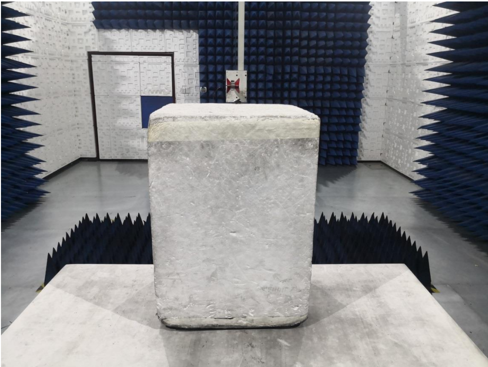
RADIATED EMISSION TEST SETUP ABOVE 1GHz
