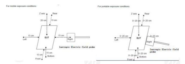
Note: Measurements should be made from all sides and the top of the primary/client pair, with the 20 cm-0cm measured from the center of the top, and 20cm-0cm measured from the center of the rest.
