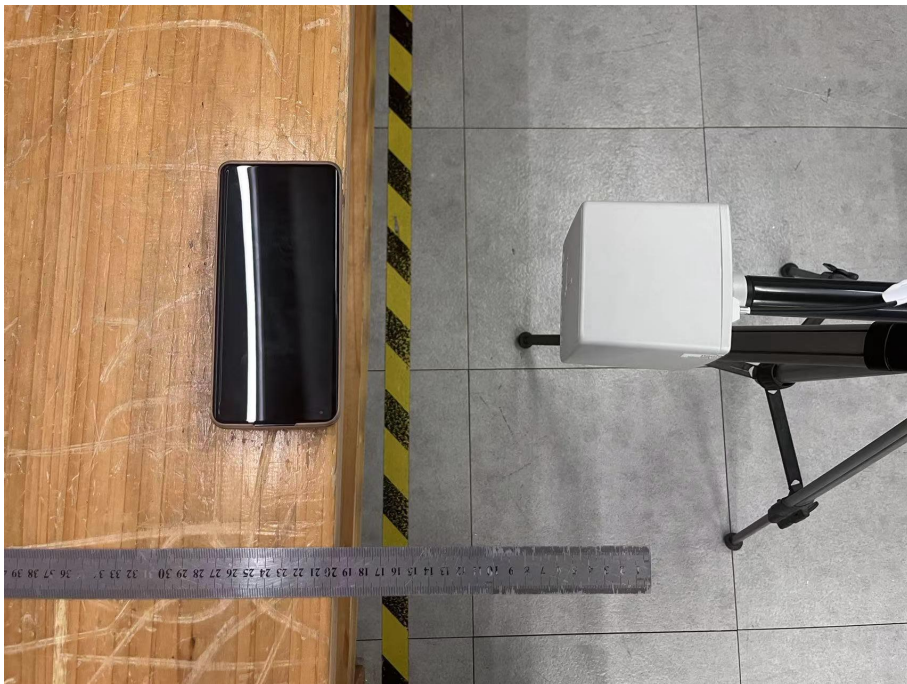
Test Position B-20cm from the edge of EUT to the geometric center of the probe
