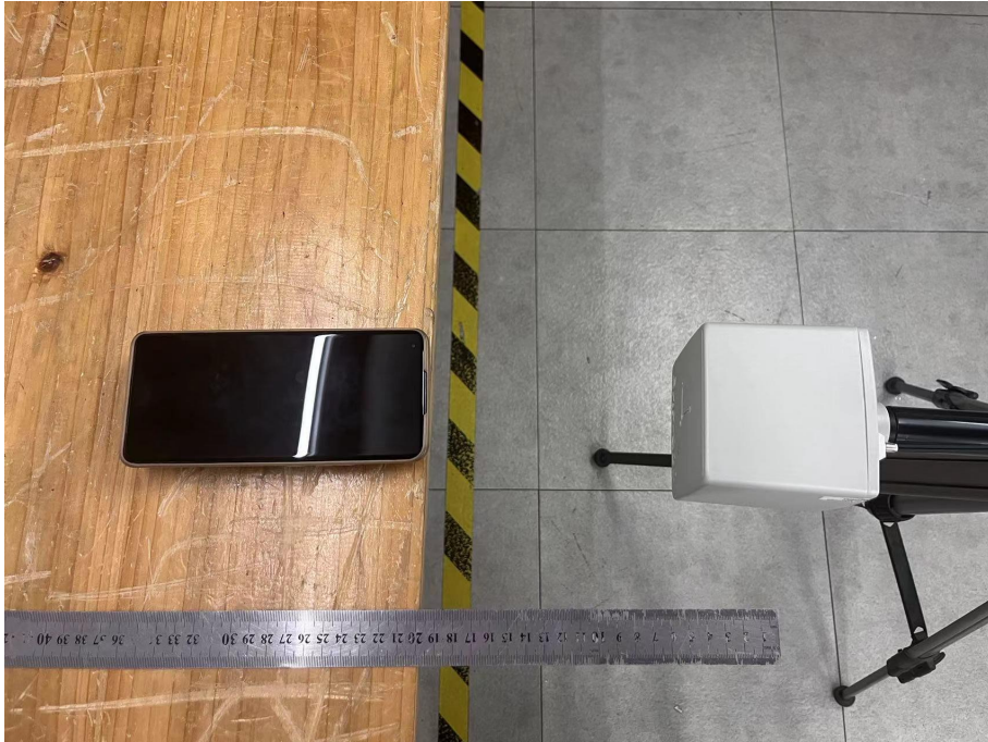
Test Position A-20cm from the edge of EUT to the geometric center of the probe
