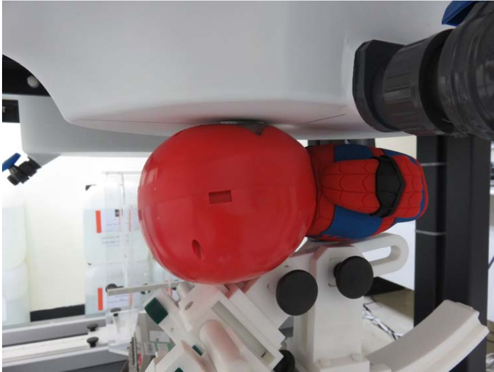
Figure 1 – Front surface with 0mm Separation
