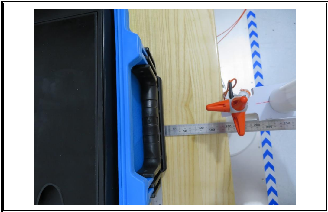
E-FILED STRENGTH MEASUREMENT SETUP FOR A POINT
