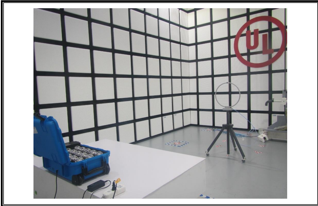
E-FILED STRENGTH MEASUREMENT SETUP FOR A POINT
