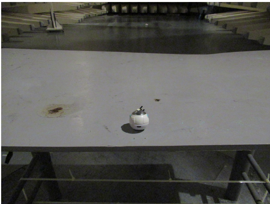
Setup for Radiated Emission
