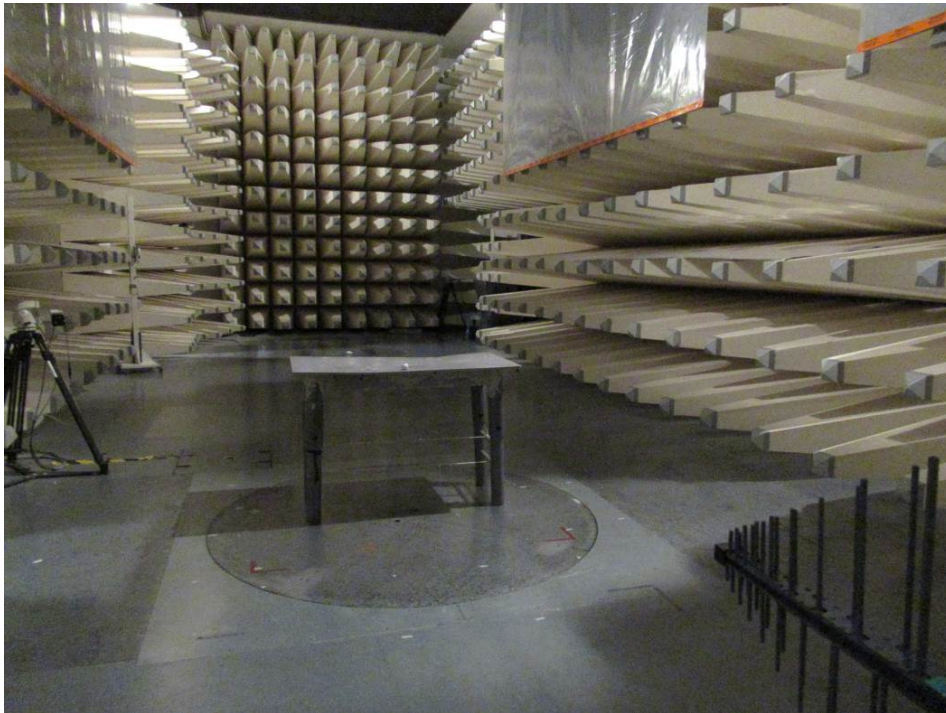
Setup for Radiated Emission
