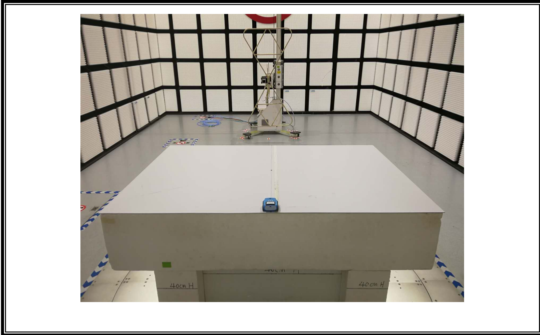
RADIATED RF MEASUREMENT SETUP (Below 30MHz)
