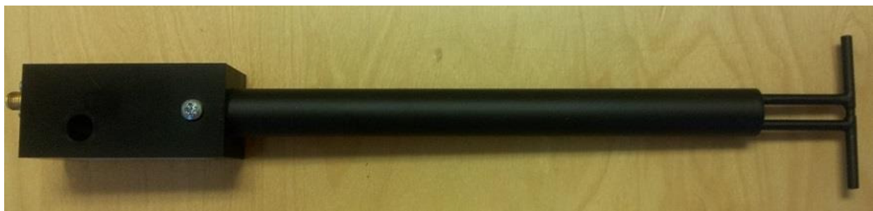
Figure 1 – MVG COMOSAR Validation Dipole
