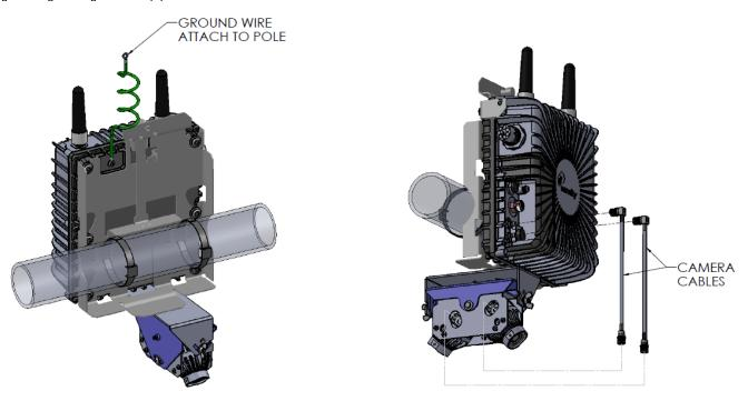
7. Connect the Video Node to the power source either onto an External Core Node or the luminaire. A T-splitter may need to be deployed). Use the delatching tool to remove the cap on the connector of the power source (External Core Node or luminaire). Connect the Video Node and the mating connector using the power cable. Press the cable firmly into the connector to ensure the connector tabs are fully latched.
