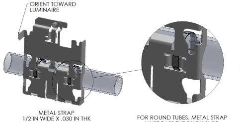
FOR ROUND TUBES, METAL STRAP MUST PASS THROUGH SLOT.
