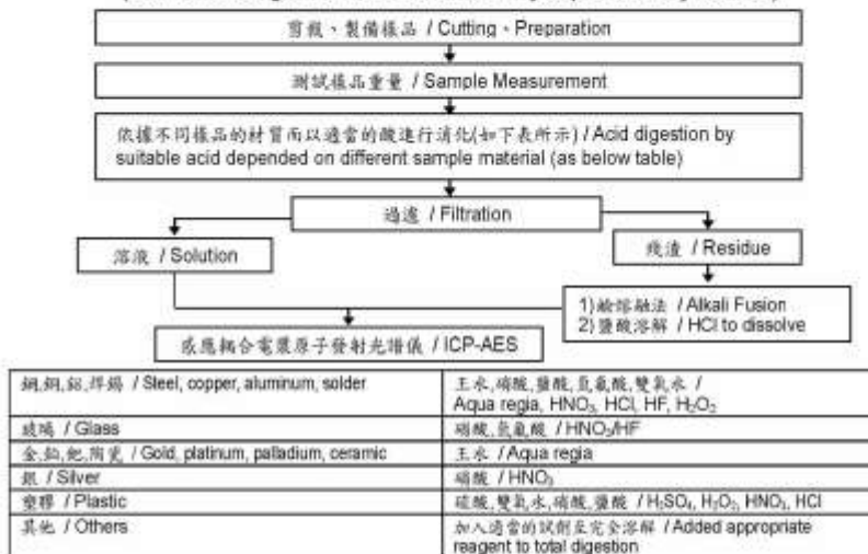
元素以 ICP-AES 分析的消化流程圖 (Flow Chart of digestion for the elements analysis performed by ICP-AES)
