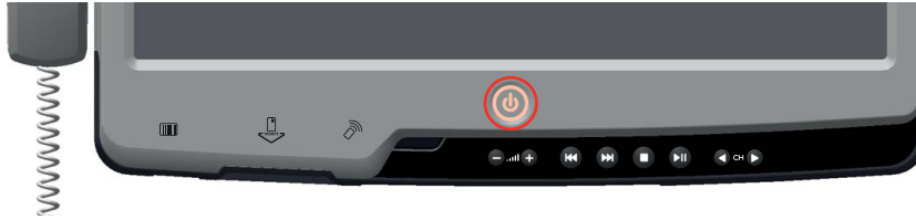
Image 3-3 Switching on the power
