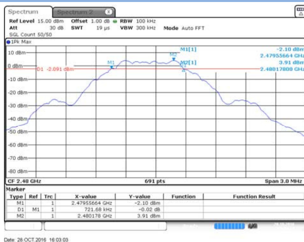
GFSK (BLE) HIGH CHANNEL
