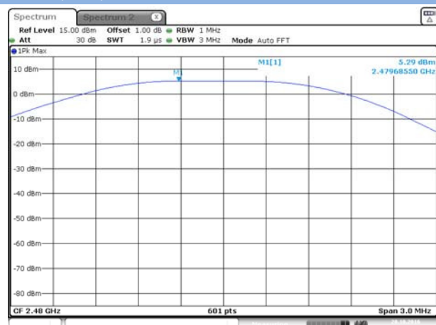
GFSK(BLE) HIGH CHANNEL
