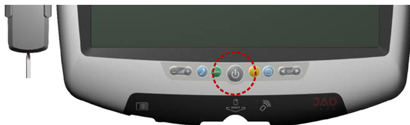
Figure 2.7: Switching on the power
