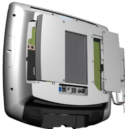
Figure C.1: Disassembling the plastic rear cover of the Zivo Unscrew the screws that secure the plastic rear covers, and then remove the covers
