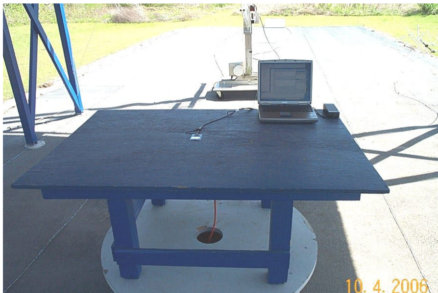
Radiated Emission Test Setup- Front
