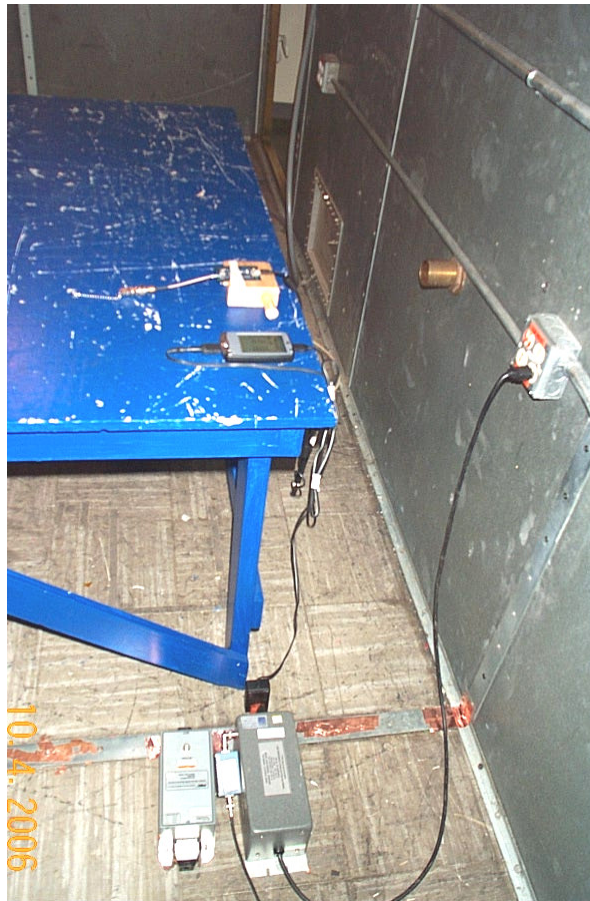
Conducted Emission Test Setup with Antenna Load
