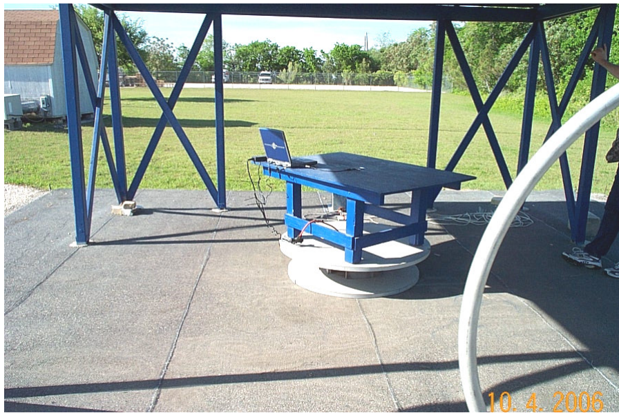
Radiated Emission Test Setup- Low Frequency Back
