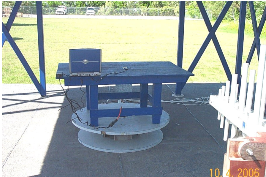
Radiated Emission Test Setup- Back
