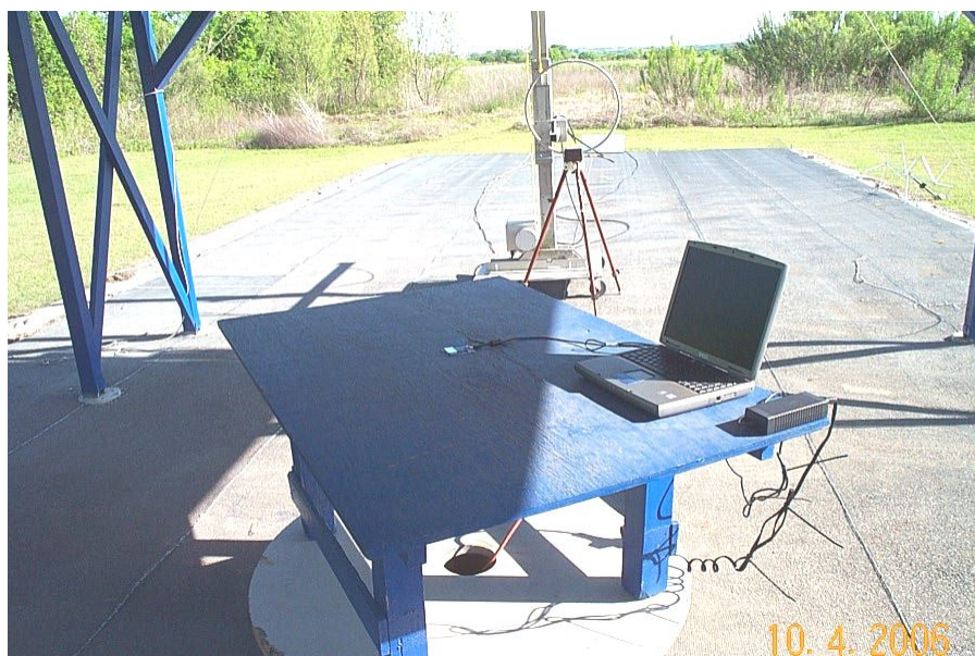
Radiated Emission Test Setup- Low Frequency Front
