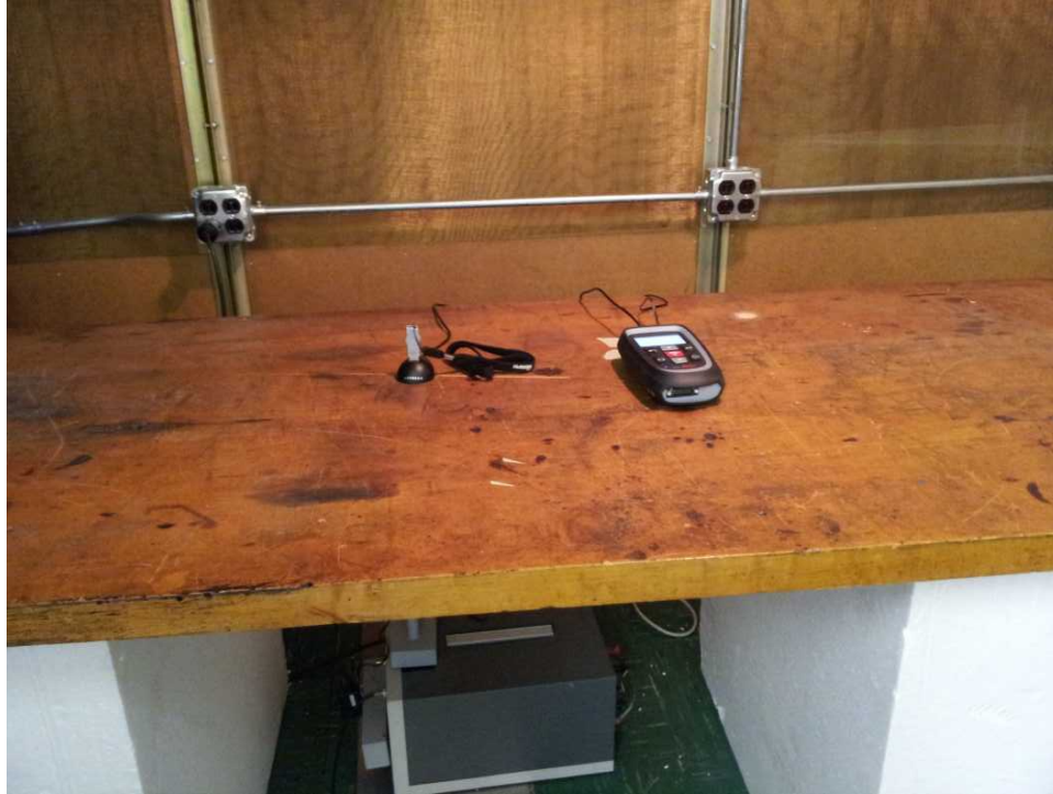
Figure 6: Conducted Emissions Test Setup Photograph(s).
