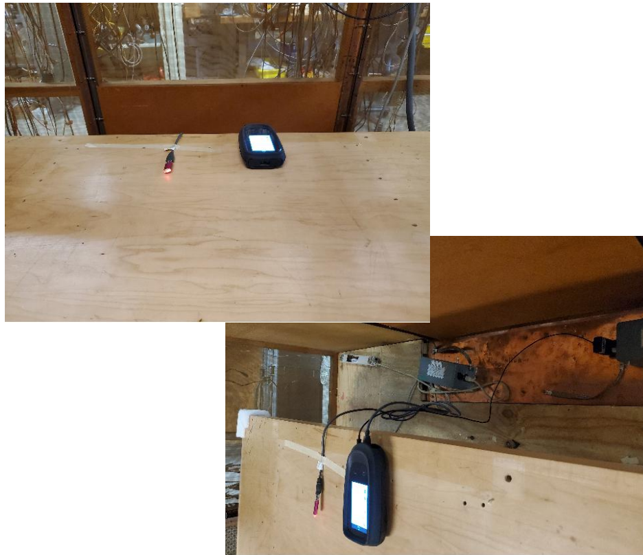
Figure 6: Conducted Emissions Test Setup Photograph(s).
