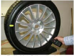
To "initiate" the wheel sensor, hold tool against the tire and rim nearest the valve stem.
