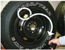
Ford 06 with Banded sensor: Hold the tools against the sidewall, 180° from the rubber stem as shown.
